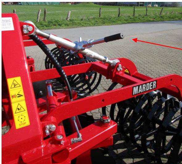
Lever for depth setting of the discs
