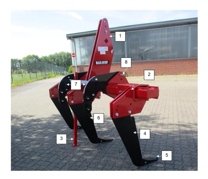
The MAULWOLF deep spade is connected to the tractor's three-point lever (1).
